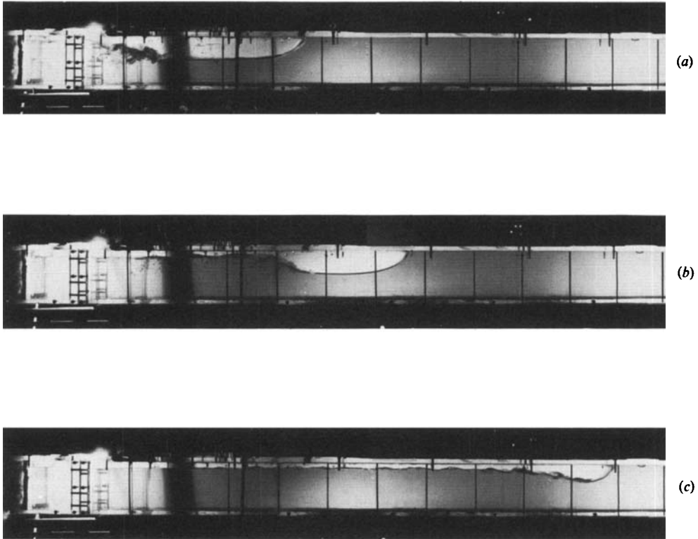
FIGURE 2. Sequential photographs of the collapse of an air cavity at \frac{2}{3} , \frac{4}{3} and \frac{5}{3} s after release, with D = 10 cm, d_0 = 0 cm, X_0 = 40 cm. These cavity shapes are representative of cavity flows with 0 \leq d_0/D \leq 0.3 .
